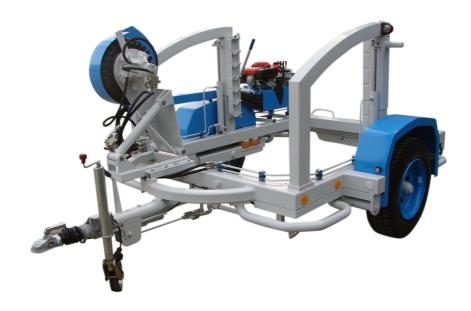
Hydraulic rewinding machine specially developed for drum carriers of the LTV-R series
